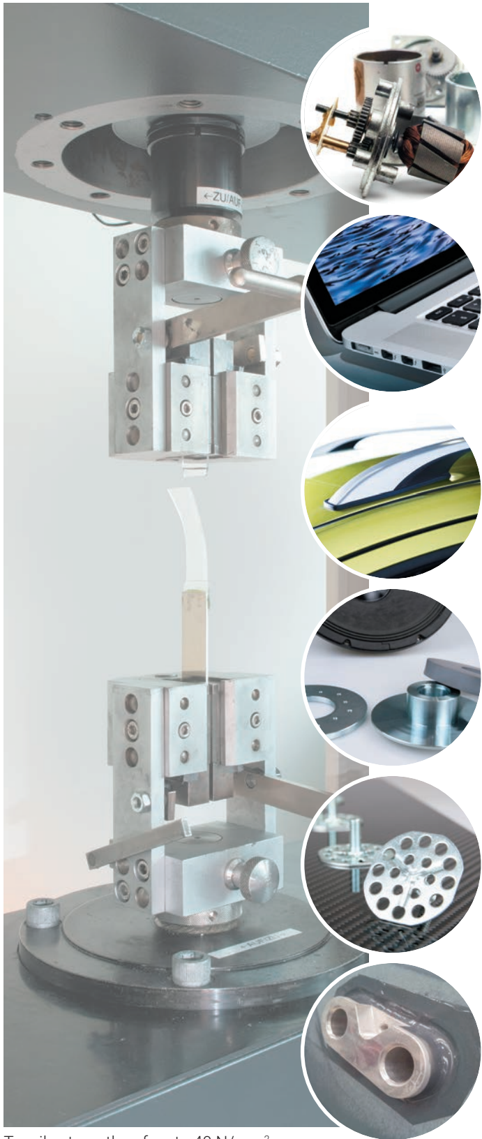
Tensile strengths of up to 40 N/mm 2 are possible with structural adhesives.
