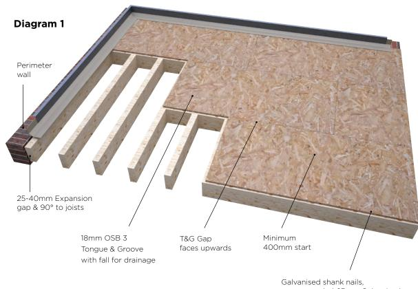
Galvanised shank nails, recommended 63mm Galvanised shank nails, spaced 200mm apart with a powered nail gun
