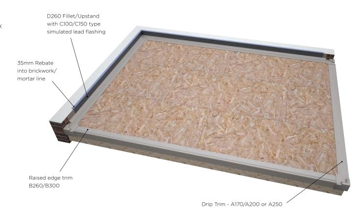
**Step 3** Apply the 75mm woven glass edging tape with catalysed TekGuard Flexi-GRP. Approximately half on the trim edge and half on the OSB 3, in preparation for the TekGuard Flexi-GRP and fibreglass layer. (See diagram right).
